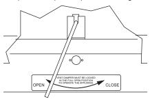
Figure 38 - Opening Vent Damper
